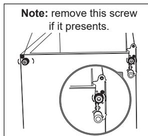
4. Unscrew and remove the bottom hinge pin, turn the bracket over and replace it.
