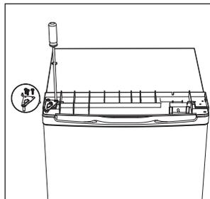
12. Put the top cover and fix it with 2 screws on the back.
