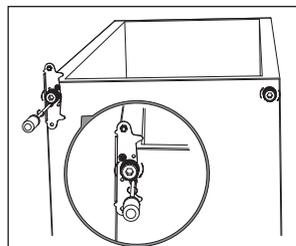
11. Place the door back on. Ensure the door is aligned horizontally and vertically, so that the seals are closed on all sides before finally tightening the top hinge.
