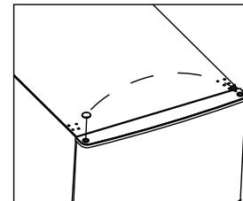
5. Unscrew the middle hinge and then lift the bottom door and put it on a soft pad to avoid scratch.
