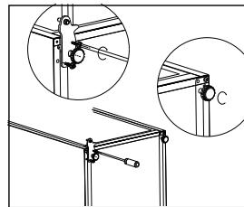
10. Stand up the unit and put the door on the bottom hinge.
