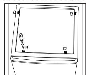
2. Unscrew the top hinge with a philiphs screw driver.
