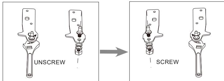
9. Install the hinge at left side and foot base at right side.
